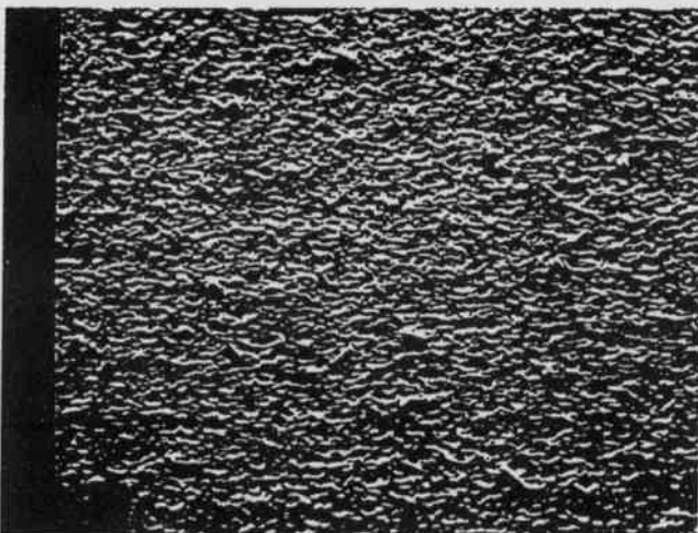
Figure 2. SEM of a cleaned titanium square at 200 x.
